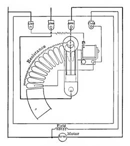
FIG. 151. Starting box for d. c. shunt motor.
